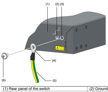
Figure 3-11 Connect the PGND cable to the grounding hole of switch
